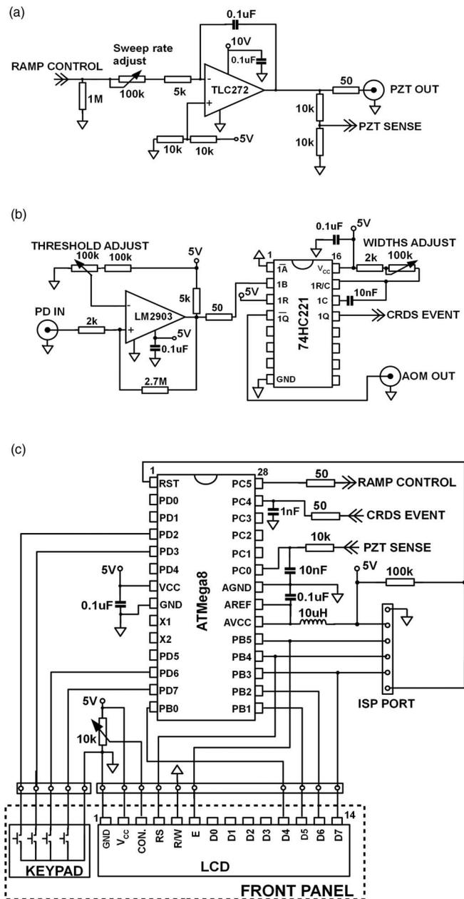
FIG. 2. Circuit diagrams of the tracking electronics sub-units: (a) ramp generator, (b) threshold generator, (c) CPU microcontroller unit.
