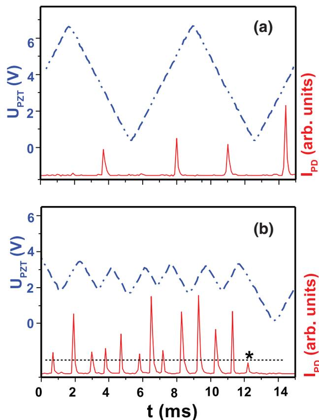
FIG. 5. Demonstration of the servoloop performance. PZT voltage (dashed line) and photodiode signal (solid line) for (a) the full sweep mode and (b) the tracking mode, respectively. The fine-dashed line in the locked mode indicates the ringdown event threshold level. Resonance marked with asterisk (\*) does not reach this threshold and thus the PZT ramp direction does not change and the lock is temporarily lost.
