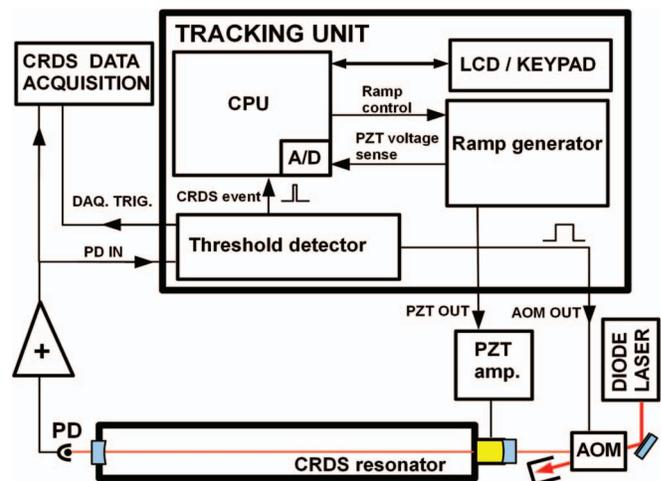
FIG. 1. Schematics of the tracking unit integration into a cw-CRDS experiment.
