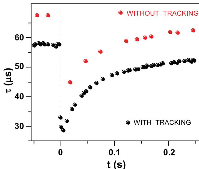
FIG. 6. Demonstration of data acquisition rate increase using the resonance tracking unit in laser photolysis experiment. Kinetics data recorded with (a) full sweep mode, (b) the tracking mode, respectively.
