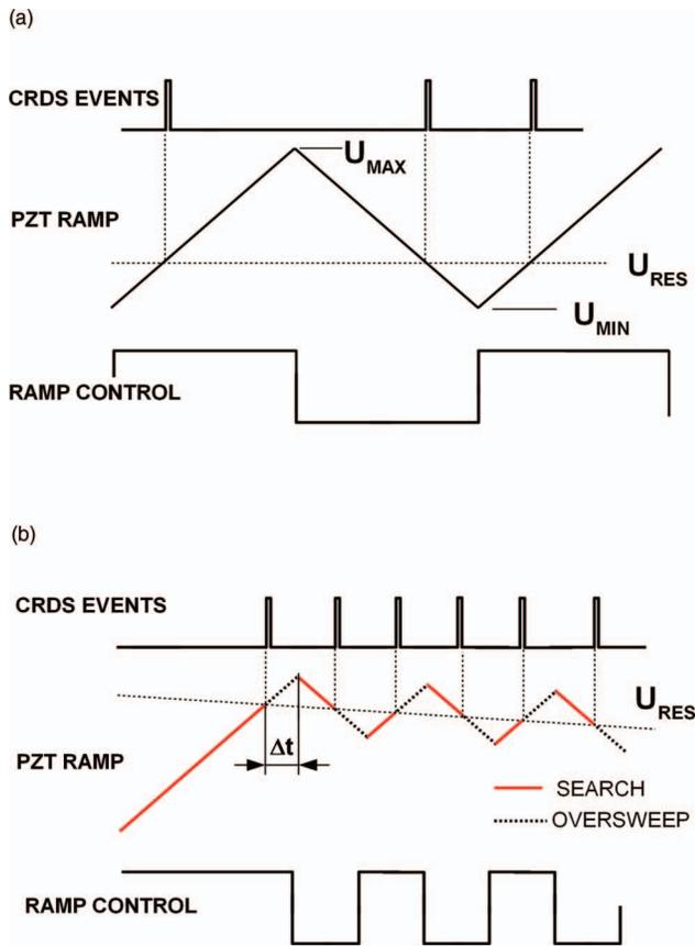
FIG. 3. Tracking unit timing diagrams for (a) the full sweep mode and (b) for tracking mode. See text for details.
