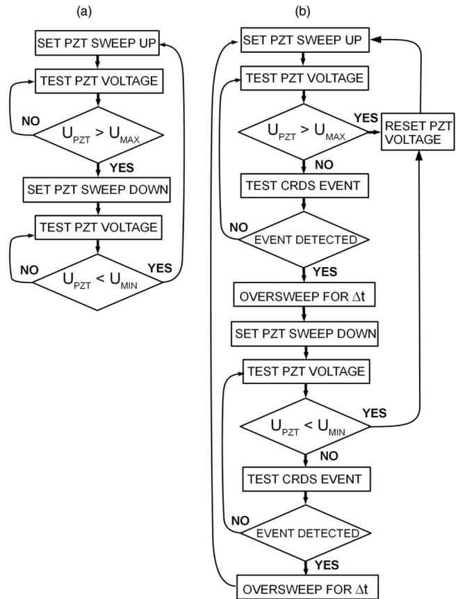
FIG. 4. Logical flowcharts of software implemented in the microcontroller to perform the full sweep (a) and tracking (b) modes as introduced in the diagrams of Figures 3(a) and 3(b), respectively.
